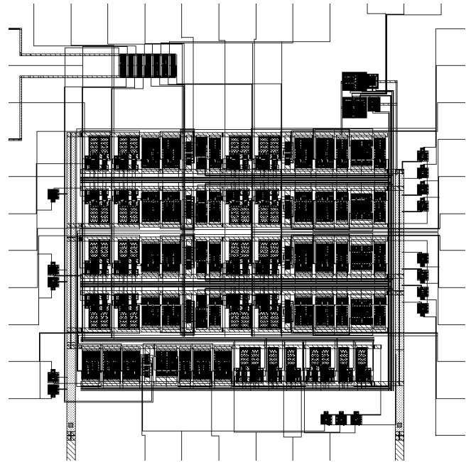
Figure 7: The 4-tap FIR-LMS adaptive filter layout.
